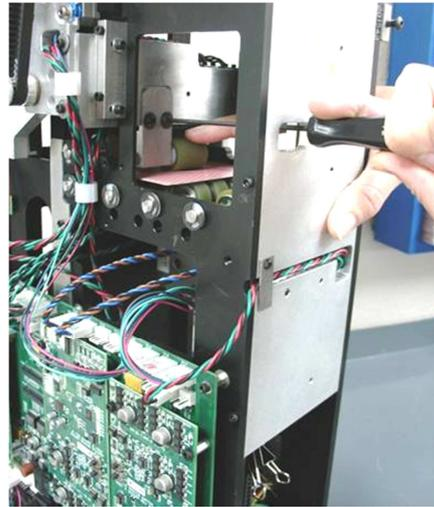
**NOTE:** Do not apply pressure to the top of the Brake Roller Block. The Assembly will tip to one side, allowing only one edge of the Brake Roller to contact the cards.
