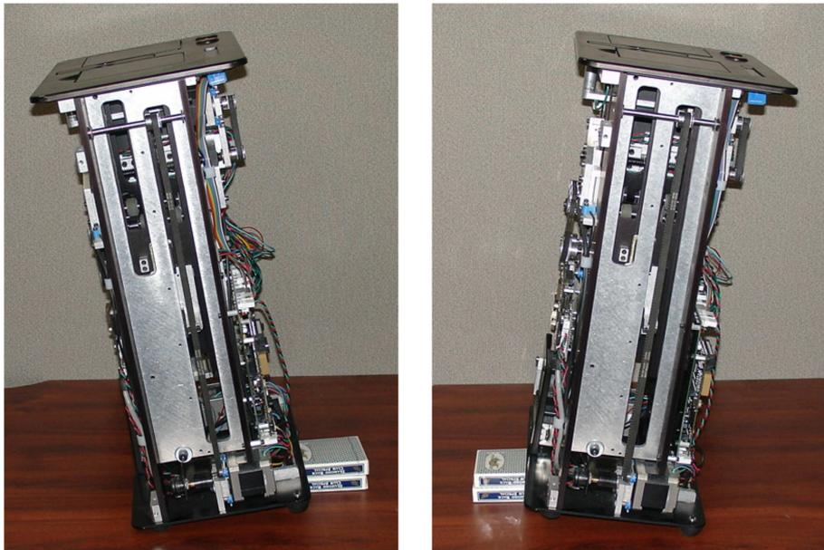
If the cards catch on the gripper pads during the lean test, mechanical travel of the gripper arms will need to be increased. Remove the two shoulder screws holding the Gripper Block with the plastic ACME threaded nut. Rotate the block  $\frac{1}{4}$  turn clockwise and re-install the shoulder screws. It is not necessary to loosen the clip that holds the ACME Nut into the block. Center the gripper assembly in the frame using Fixture F1099.
